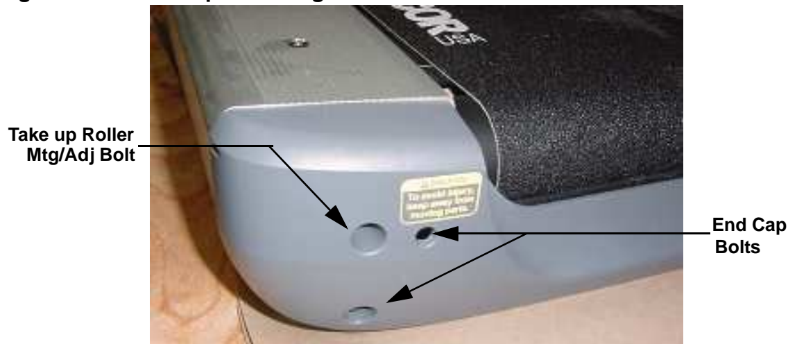
Diagram 6.7 - End Cap Mounting
